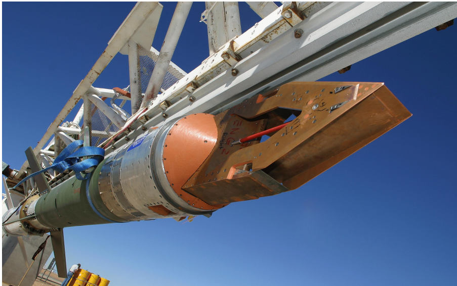
Figure 1: The UQ scramjet mounted on the Terrier Orion sounding rocket. Photo: Chris Stacey, The University of Queensland
